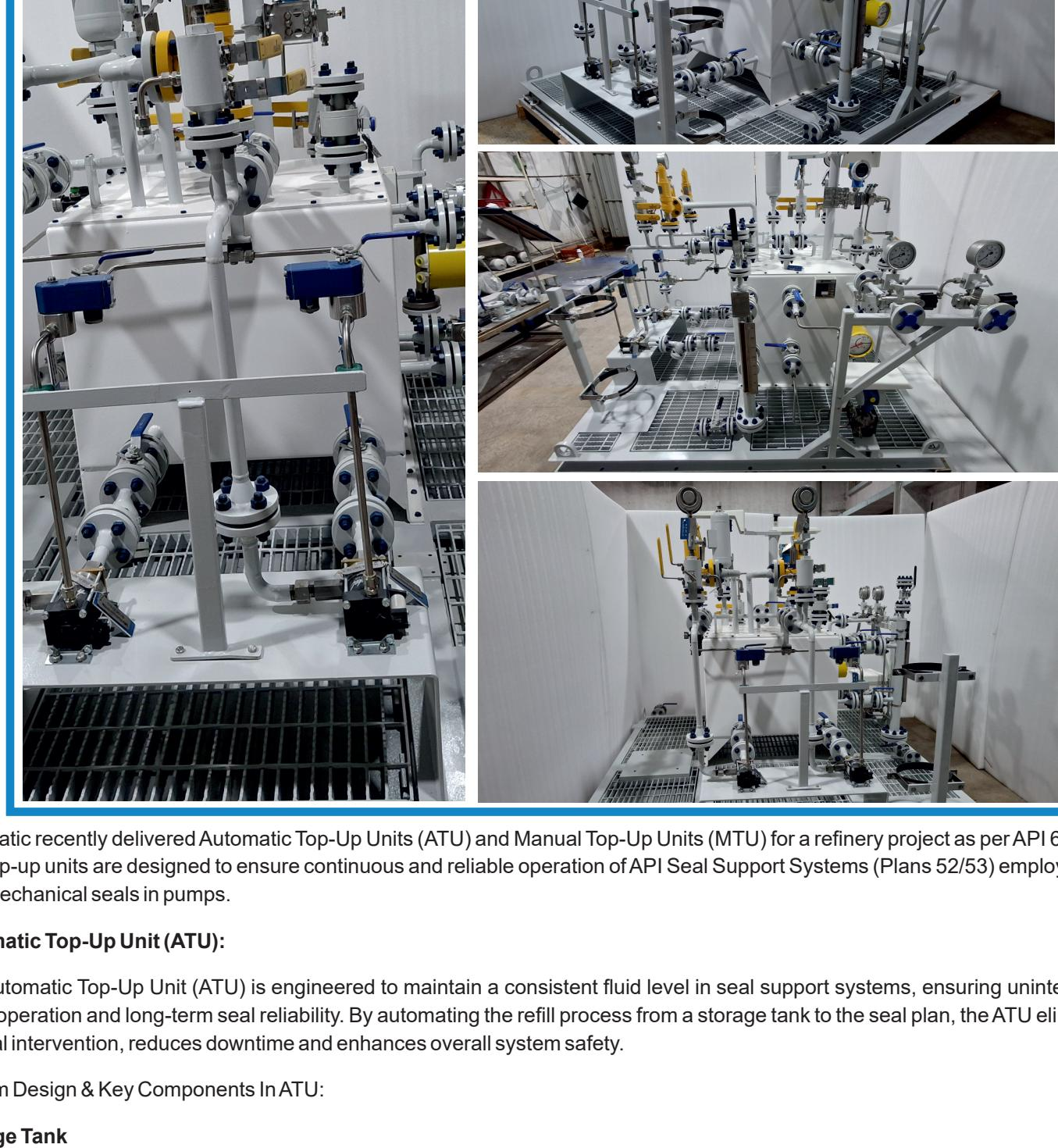
Sealmatic recently delivered Automatic Top-Up Units (ATU) and Manual Top-Up Units (MTU) for a refinery project as per API 682. The said top-up units are designed to ensure continuous and reliable operation of API Seal Support Systems (Plans 52/53) employed with dual mechanical seals in pumps.
